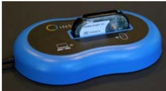
Figure 6.3. Electronics Module connected to the Smart Cable.
