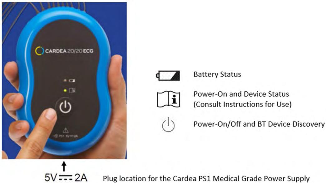
The Battery Status LED operation is described in the next section, Rechargeable Battery Operation. The PS1 Medical Grade Power Supply plugs into the end of the ECG Transmitter, as indicated above. Fully charge the ECG Transmitter before initial use.
